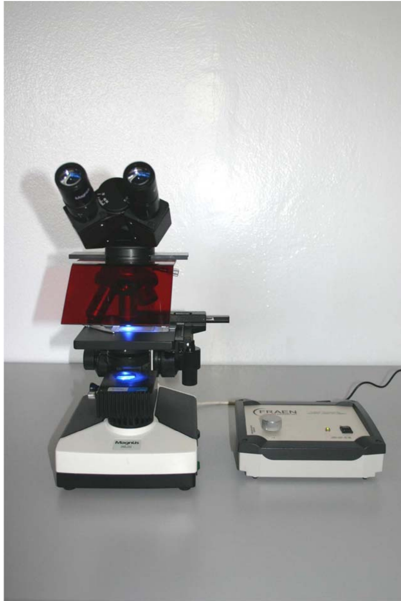
MLXi microscope with MicroLED fluorescence illuminator installed.
